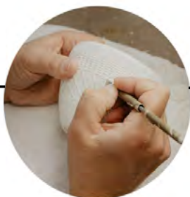
Realization of the plaster model
